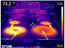
The range elements were operated with indicator set to HIGH until the element was noted to be fully red or until a defect was noted. The unit calibration was not verified. If the client would like to verify temperature calibration, an appliance specialist should be consulted.
