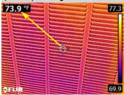
Thermal image of the temperature variance between the return/supply air for the main floor AC condensing unit. The temperature variance between the return/supply air was 11.7 degrees(F). This variance was less than typically expected, a complete evaluation by an HVAC contractor is needed.
