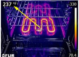
The oven elements were operated with indicator set to HIGH until the element was noted to be fully red or until a defect was noted. The unit calibration was not verified. If the client would like to verify temperature calibration, an appliance specialist should be consulted.
