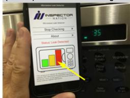
The microwave was tested for leakage at the door area during operation. The test indicated leakage above what is considered safe or normal. An appliance repair specialist should be consulted for further evaluation and repair to ensure safe and proper operation of the appliance.
